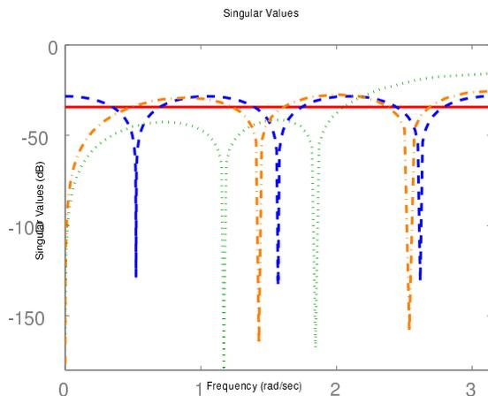
**Fig. 3.** Magnitude plot of  $E(z)$ :  $H^\infty$  optimal IIR (solid),  $H^\infty$  optimal FIR (dash), CLSD [7] (dash-dots), and KWA [8] (dots).
