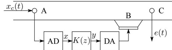
Fig. 1. Active noise control system
