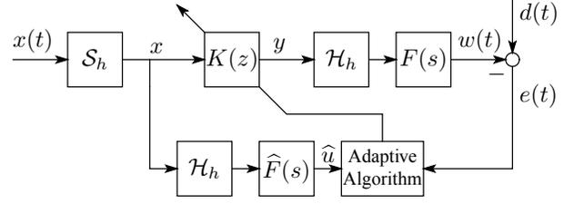
Fig. 3. filtered- $x$  adaptive system
