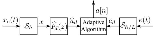
Fig. 4. filtered- $x$  adaptive scheme
