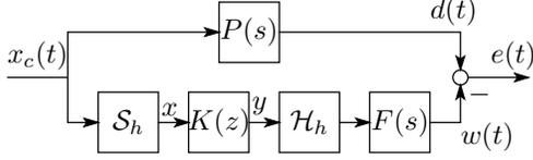
**Fig. 2.** Block diagram of active noise control system
