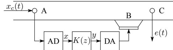
Fig. 1. Active noise control system
