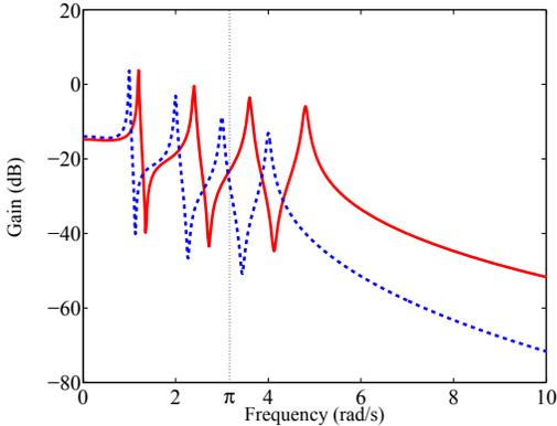
Fig. 5. Frequency response of  $F(s)$  (solid) and  $P(s)$  (dash). The dotted line shows the Nyquist frequency.
